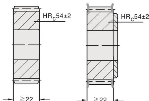
Fig. 4: Design of Connecting Components
