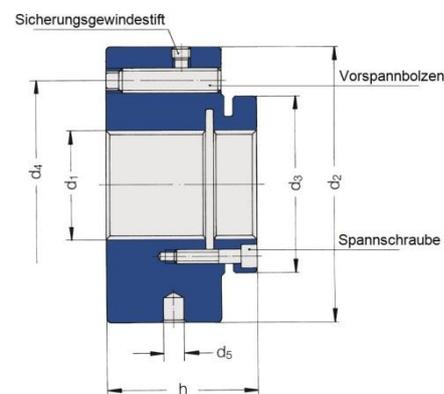
Fig. 3: Sectional view Spieth locknut > M80
