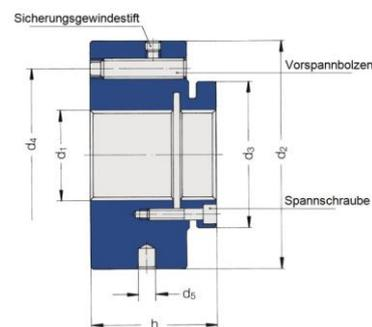
Fig. 5: Sectional view of Spieth locknut > M80
